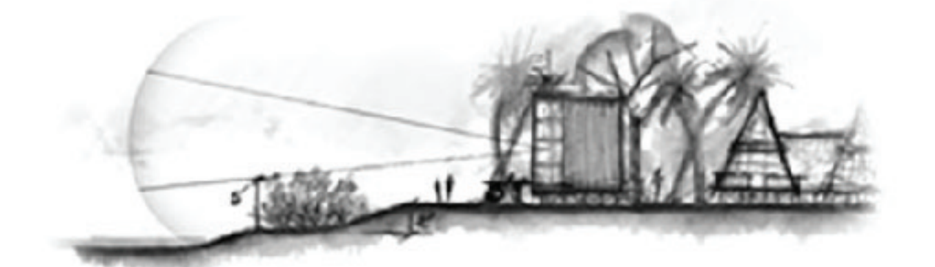
For having a natural green barrier of kheyah tree in between the sea and the site, the whole structure is elevated 3' from ground to ensure the sea view from the rooms
